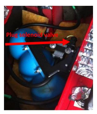
Disconnect the original connector on the solenoid valve and connect it to the matching connector of the control system. Then put the second connector of the control system on the solenoid valve:
