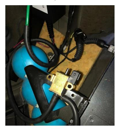
Attach the control system as shown in the picture and fix them with self-adhesive Velcro fasteners on the car body:
